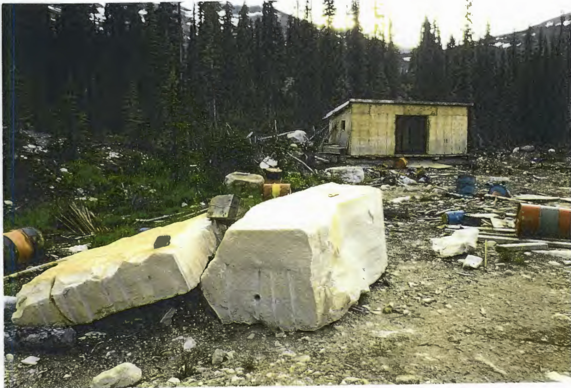
Figure 4.15. Quartzite blocks quarried at the Wishaw Lake site. Those particular blocks are not in the size range preferred by industry ( 1.4 x 1.6 x 3 m )
